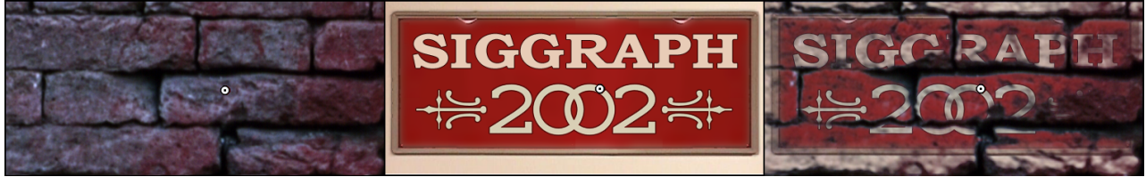
Figure 3 Similarity Cloning: (left) original texture, (center) cloning texture, (right) single point cloning. Strength = 75%, Distance = 500K, d = 5 , Levels 0,1.
