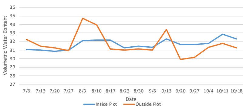
Figure 2. Available Moisture Inside and Outside Test Plot Osage County 18 inches below surface
