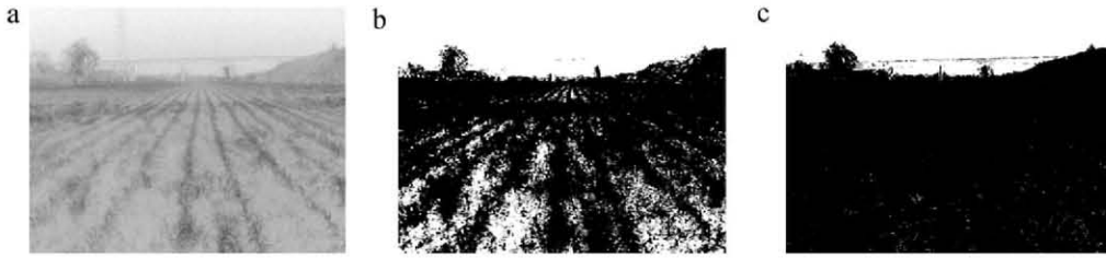
Fig. 6. (a) ExB image computed through Eq. (5); (b) binary image obtained by applying the mean histogram; (c) binary image obtained by applying the Otsu's approach.
