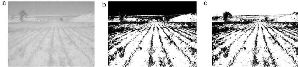
Fig. 7. (a) ExR image computed through Eq. (4); (b) binary image obtained by applying the mean threshold; (c) differences between binary images given in Figs. 6(c) and 7(b).
