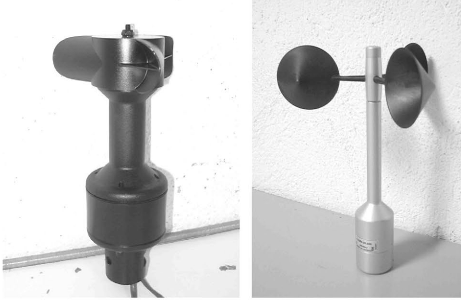
Figure 7. NRG IceFree anemometer (left) and Thies 4.3350 anemometer.
