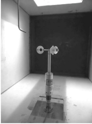
Fig. 6. Climatronics 100075 anemometer placed in the S4 wind tunnel of the IDR/UPM Institute, to carry out a calibration equipped with a porous-cups rotor (left). Anemometer output signal, V_{\text{output}} , measured in one turn (right-top). Relative-to-the-average rotational speed, \omega/\omega_0 , calculated in that turn (right-bottom). T is the period of the anemometer's rotation [15].
