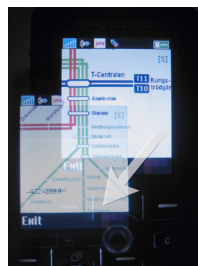
Figure 4. Two superimposed images illustrate the implemented "Peephole" interaction technique. A small tracked display acts as a viewport into a larger virtual display and by moving the device the user is able to view different portions of the virtual display.
