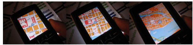
Figure 3. Zooming in the navigation guide. As the user positions the device on top of a subway station on the map, a local road map becomes available and the station's name can be played back through the earphones. The user can interact with the map by lifting the device away from the surface to zoom out in the region, or by lowering it to zoom in.
