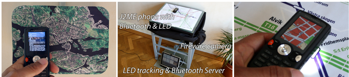
Figure 1. The LightSense system tracks the LED on commercial cell phones, enabling them to be used as spatially aware handheld devices. The outside-in approach tracks the light source and streams the data to the phone over Bluetooth. a) A wall-mounted map with embedded light sensors provides hotspot tracking. b) A table-top setup tracks the phone with a camera through a diffused glass surface. c) The spatially aware device augments a physical map with a detailed interactive road map of the area of interest.
