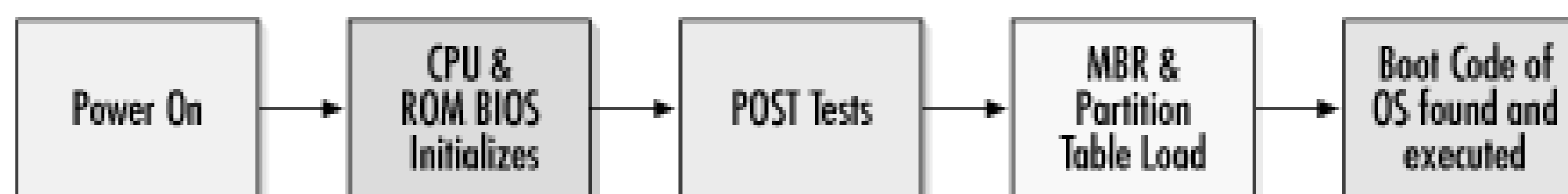
Figure 2-1. Normal PC boot sequence (regardless of operating system)
