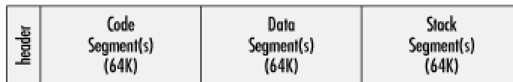
Figure 2-5. Simplified structure of an .EXE file
