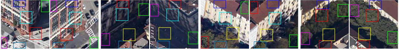
Figure 10. Image pairs from ‘aerial’, matched with Hybrid++. The overlaying boxes indicate patch proposals. Red boxes denote patches that do not match, according to MatchNet. Boxes with colors other than red indicate matches, with the color encoding the correspondence.
