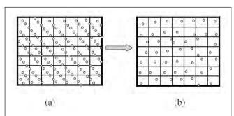
Figure 3. Pseudo-grid for surface initialization: (a) Original scanning points, and (b) Points on the initial surface model.
