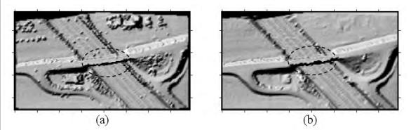
Figure 11. Shaded relief map of sample 15: (a) Initial surface model, and (b) Generated DEM including a land bridge.
