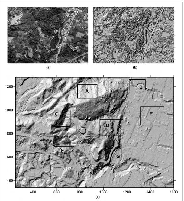
Figure 12. Test site in the mountainous area: (a) Aerial image, (b) Initial surface model, and (c) Generated DEM with seven reference samples (squares A to G).
