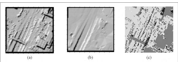
Figure 9. Shaded relief maps of sample 4 (buildings, crossover bridge and gangway): (a) Initial surface model, (b) Generated  $_{\rm DEM}$  excluding the crossover bridge, and
