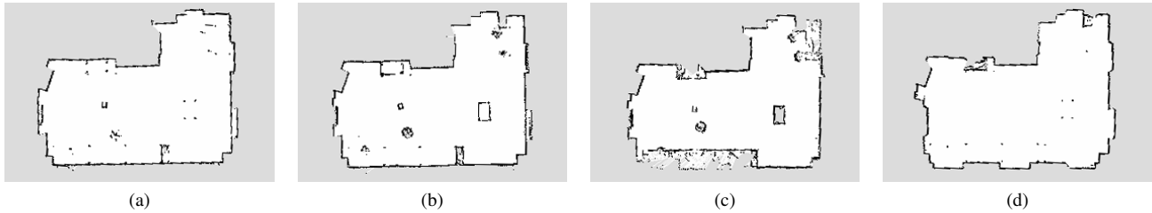
Fig. 7: Traversability map for an office-like scenario: (a) PFF, VLP-16 and robot height = 25 cm, (b) PFF, VLP-16 and robot height = 40 cm, (c) PFF, VLP-16 and robot height = 100 cm and (d) Hokuyo 2D LiDAR.
