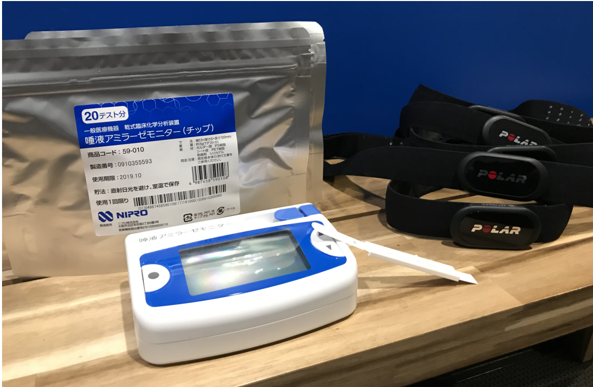
Figure 1: Data collection equipment. Left: pouches of saliva swabs. Center: point-of-care salivary amylase meter, with a single saliva swab. Right: Polar H10 cheststrap heart rate monitors.
