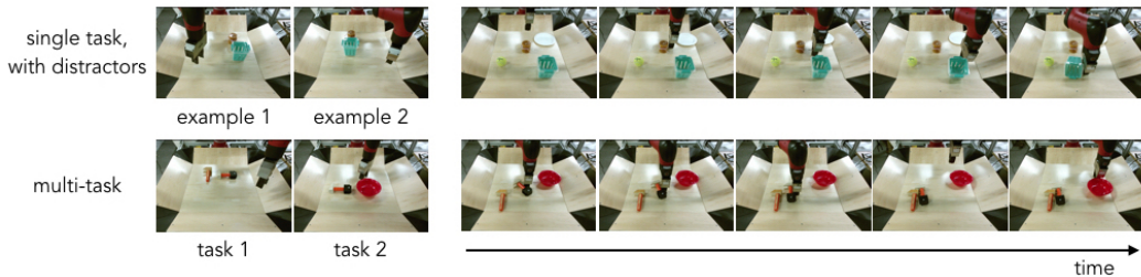
Figure 3: Object arrangement performance of our method with distractor objects and with two tasks. The left shows a subset of the 5 positive examples that are provided for inferring the goal classifier(s), while the right shows the robot executing the specified task(s) via visual planning.
