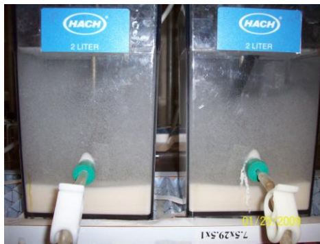
Flocculation Process Jar Test Calibration
