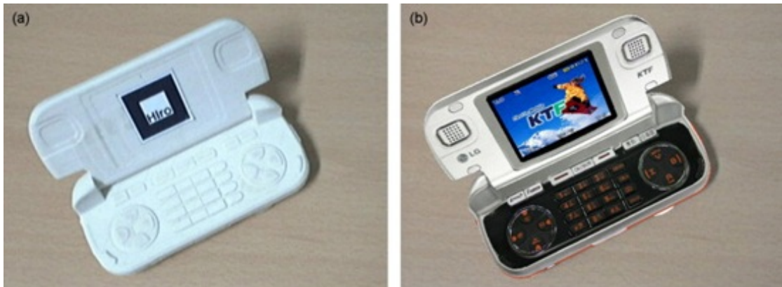
Figure 2.6: (a) Physical model with AR marker (b) augmented as a game phone [Park et al., 2009]
