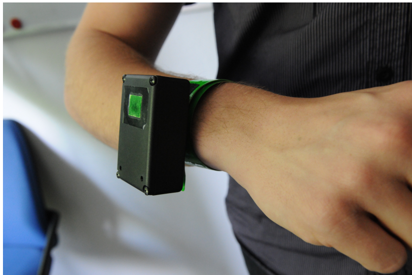
Figure 8.11: The electronic triage tag is attached to a colored bracelet, which closes automatically when snapped against an arm.
