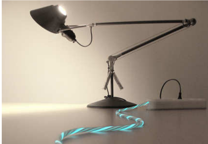
Figure 3.2: The Power-Aware Cord shows how much energy the connected lamp consumes [Gustafsson and Gyllenswärd, 2005].
