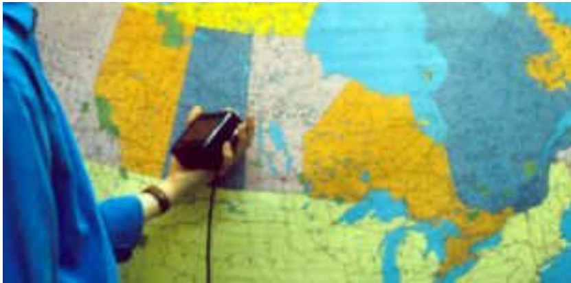
Figure 2.2: Weather information is shown for the region the handheld device is currently pointing at [Fitzmaurice, 1993].
