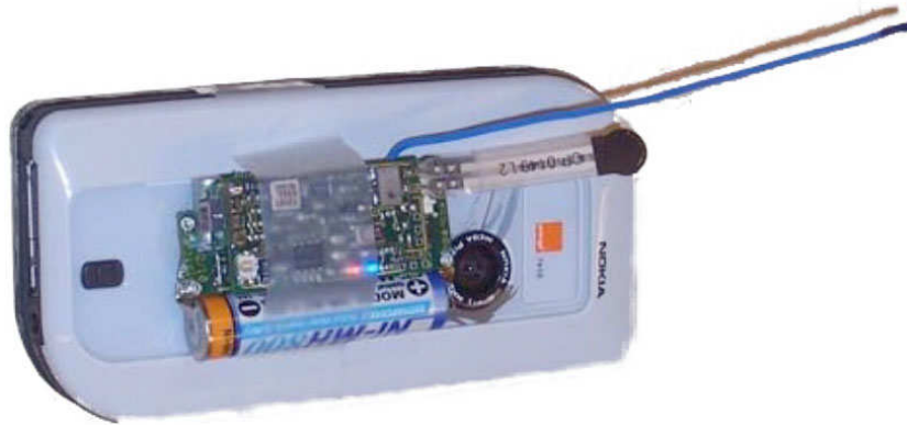
Figure 2.9: A mobile phone is augmented by sensor hardware [Ballagas et al., 2007].
