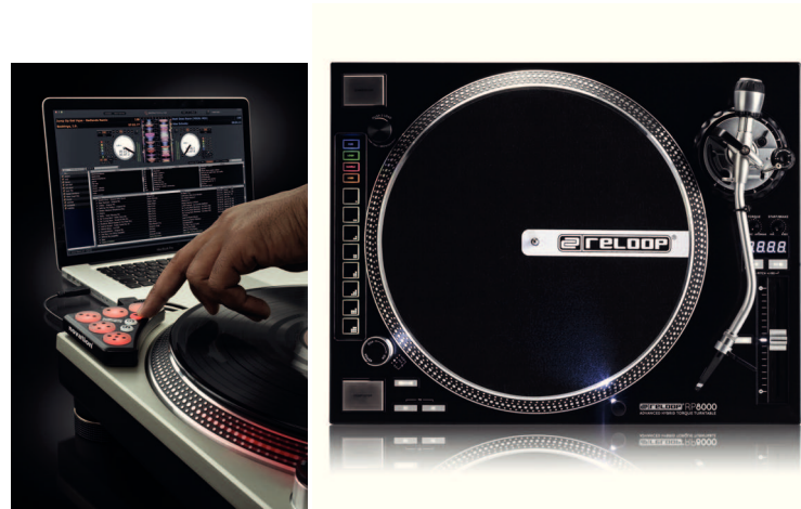
Figure 3.10: Left: The Novation Dicer MIDI controller for DVS (Image courtesy of Focusrite). b) The Reloop RP-8000 turntable with integrated buttons to control the host DVS software (Image by Reloop)
