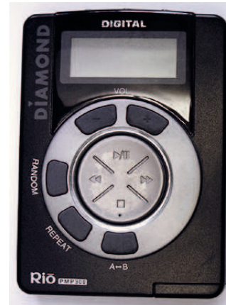
Figure 2.1: The Diamond Rio PMP300 was the first commercially successful portable MP3 player. Although users were now able to carry large music collections with them, the controls were still the same as on other portable music players (Image courtesy of John Fader).
