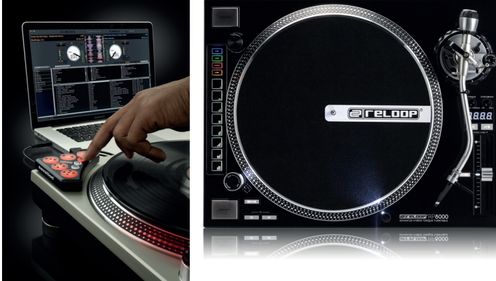
Figure 3.10: Left: The Novation Dicer MIDI controller for DVS (Image courtesy of Focusrite). b) The Reloop RP-8000 turntable with integrated buttons to control the host DVS software (Image by Reloop)
