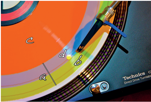
Figure 3.6: DiskPlay displaying a track. (a) Remaining playback area (blue). (b) Part already played as progress indicator (green). (c) Unused timecode part (red). (d) Cue points (yellow dots) (Taken from [Heller, Borchers, 2012]).
