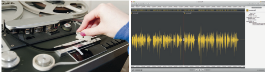
Figure 1.3: Cutting audio material in the analog and digital world. The tools in the digital workflow are metaphors of the once physical activities. (Left image from phizyx.com)
