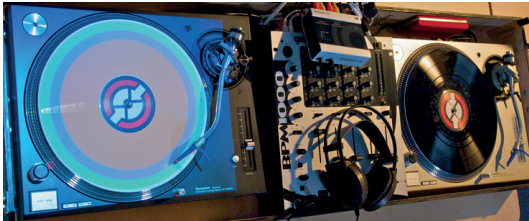
Figure 3.7: The DiskPlay test setup with the augmented turntable on the left and the traditional timecode vinyl on the right. The projector (not in the picture) is above the left turntable (Taken from [Heller, Borchers, 2012]).
