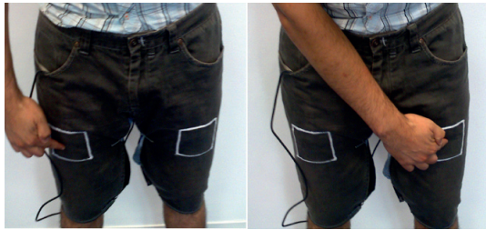
Figure 2.16: Two Fabritouch pads integrated into a pair of trousers. Users tried both parallel (left) and crossed touch gestures (right) (Taken from [Heller et al., 2014a]).
