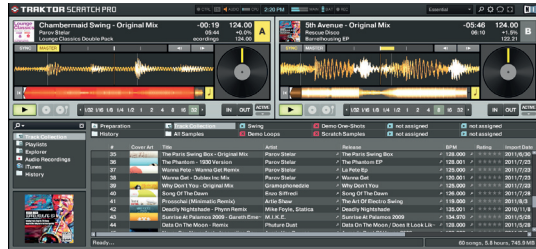
Figure 3.2: Traktor Scratch Pro user interface. The left track is close to the end, indicated by the waveform overview flashing red.
