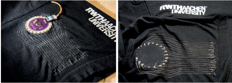
Figure 2.4: The initial Pinstripe prototype. 18 parallel lines of conductive thread are sewn into the sleeve of a T-shirt and connected to a LilyPad Arduino (Image taken from [Karrer et al., 2011]).
