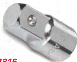
A1216 ADAPTER • 3/8" Female to 1/2" male • Overall length: 1-5/16" / 33.3mm
