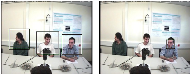
Figure 6: FGNET sequence, face pose changes: The left plot shows detections of the local context of faces while the right plot shows the output of the object-centered detector. The latter misses two faces because it is restricted to frontal view detection. While an additional specialized side-view detector could be trained (assuming the object-centered paradigm) this would at least require to gather a large amount of additional training data of profile views. Contrastingly, the local context approach does not require such specialized training and is robust to face pose changes.
