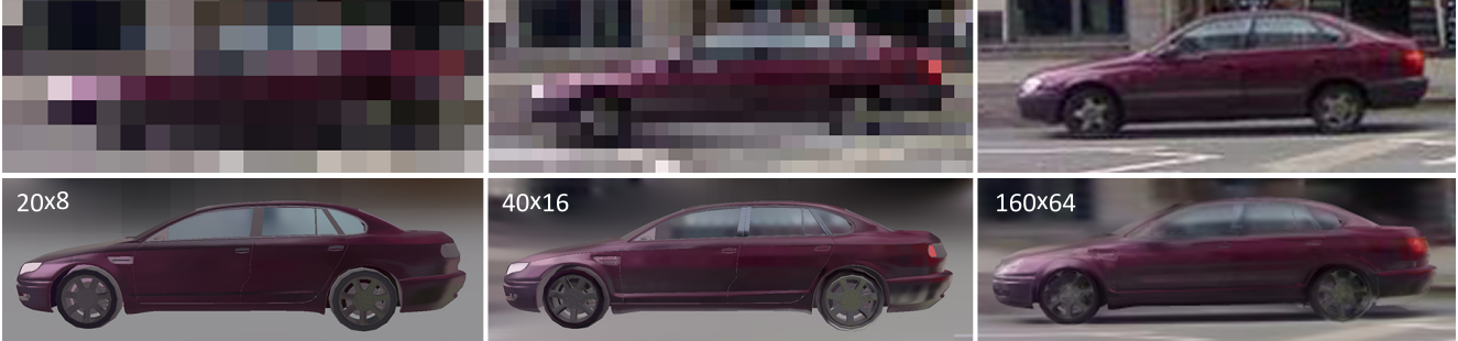
Figure 11. Super-resolution from an input image ( Top ) using our approach ( Bottom ) for three different resolutions 20 \times 8 ( Left ), 40 \times 16 ( Middle ) and the original size 160 \times 128 ( Right ). Note how even small features such as the the break light upscale to plausible structures.
