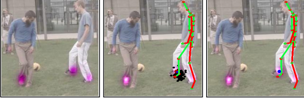
Figure 2. Refinement of the Body Part Detections using the pose posterior. Left: Overlay of the heat-map for the right ankle joint over the input image. Middle: sampling from pose posterior around the rough 2D position p_{j,c}^{init} (black dots). Right: The final refined location of the body part d_{j,c} (blue dot).
