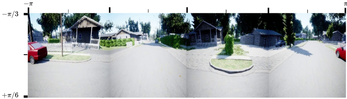
Figure 2: Generated panorama image with spherical mapping on AirSim.
