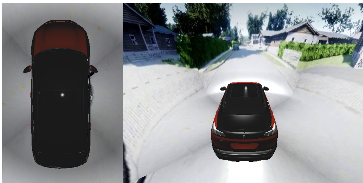
Figure 5: Generated sample 3D surround view using the bowl mesh from top and horizontal view.
