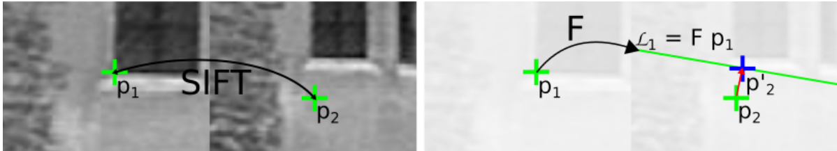
Figure 2: From an imperfect match (p_1, p_2) considered inlier by AC-RanSaC, the “perfect match” (p_1, p'_2) is constructed using p'_2 the orthogonal projection of p_2 on the epipolar line \mathcal{L}_1 = F p_1 where F is a realistic fundamental matrix given by AC-RanSaC. This does not guarantee that p'_2 represents the same physical point as p_1 , but that some 3D point at possibly different depth projects exactly at p_1 and p'_2 .
