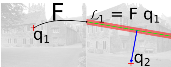
Figure 4: A random point q_1 is drawn from the left image. Using the ground truth model F , the epipolar line \mathcal{L}_1 = F q_1 is computed. Then position on this line and a distance to \mathcal{L}_1 are drawn uniformly in order to create q_2 so that it remains in the image and out of the inlier zone (marked in red) defined by the inlier noise level.
