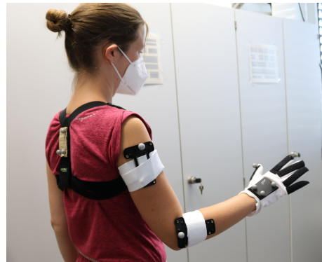
Figure 2: Stacking-scenario setup. Positions of markers attached on the arm and the back of the subject are recorded using a camera based motion tracking system.
