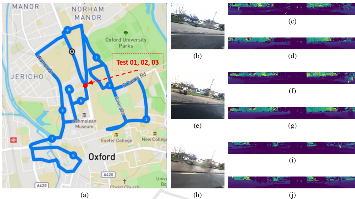
Figure 2: Three different sample tests, e.g., Test 01, Test 02 and Test 03 from Oxford Radar RobotCar outdoor dataset. (a) Satellite-view with approximated GPS positions. (b), (e) and (h) Left-view of test images obtained from Grasshopper2: cloudy, sunny, rainy, respectively. (c), (f) and (i) 3D LiDAR point clouds (intensity) obtained from Velodyne left. (d), (g) and (j) 3D LiDAR point clouds (depth) obtained from Velodyne left.
