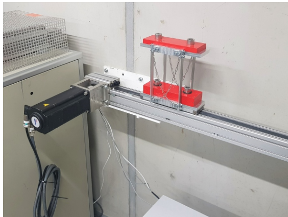
(a) Positioning stage with load on leaf springs
