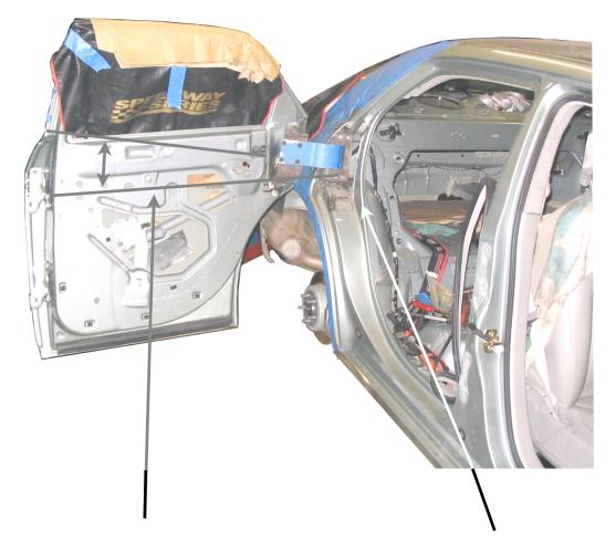
On these cars, we recommend that the hinge have a 3° to 5° angle from the side. This makes the door look more level when open and let gravity hold the door open. Be sure that the striker and latch are also angled at the same 3° to 5° to close properly.
