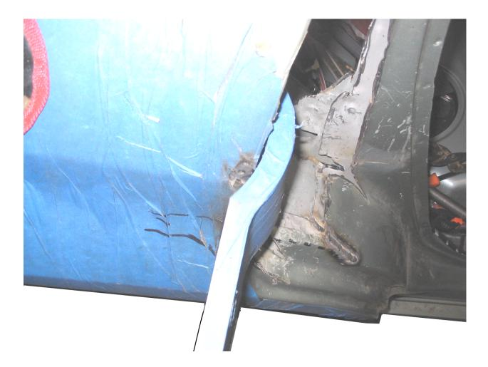
It is VERY important to "recess" the hinge in the quarter panel so that the hinge strap just clears the edge of the quarter panel skin.
