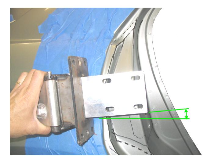
We suggest tilting the hinge up  $3^{\circ}$  to  $5^{\circ}$  when in the closed position.
