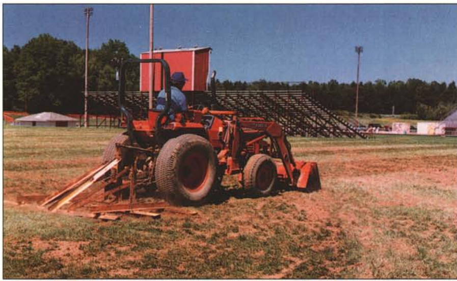
Topdressing the field, then using a level bar like this one, can even-out the contours and improve surface drainage.
