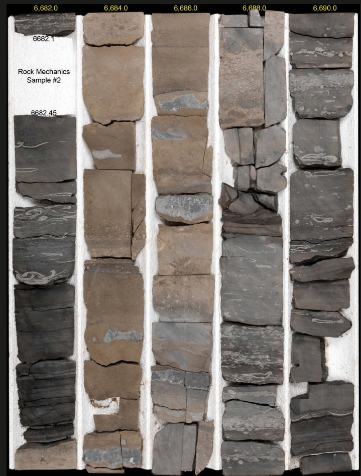
Core from the Uteland Butte Member of the Green River Formation, Uinta Basin, Utah (Bill Barrett Corp., 14-146). One of the productive horizontal targets is the roughly 5-foot-thick tan dolomitic bed with porosities ranging from 20 to 30%. The oil is sourced from the surrounding darker gray organic-rich limestones, which contain abundant shell fossils, indicating that these layers were deposited in a freshwater lake.
