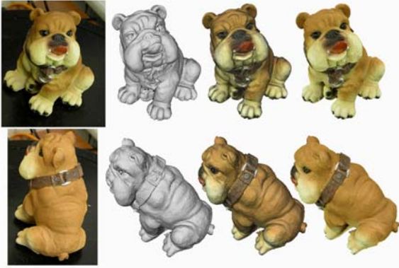
Fig. 4. An example of color mapping. The 3D model is composed by 1 million triangles, with a mapped photographic dataset of 8 images 2560 \times 1920 . From left to right: original photos, geometry, color + lambertian shading, color only.
