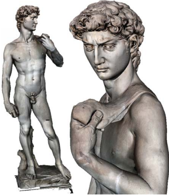
Fig. 1. A 56 million faces 3D model with color coming from a 520 Mpixel dataset (64 photos)
