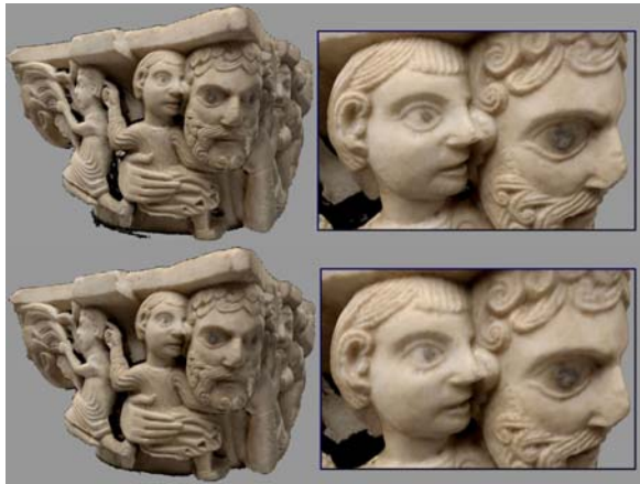
Fig. 6. Marble capital. Top row: 6 million triangles, bottom row: 1 million triangles. The photographic dataset used was 8 images 1800 \times 1200 , per-vertex mapping encoding. Even reducing the complexity of the 3D model, the mapping quality remains high; quality degradation due to the per-vertex approach starts to appear on the smaller model as we get very close to the object (the eye of the small figure is 6mm wide).
