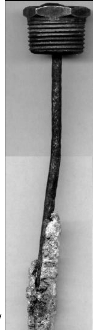
Fig 7 - Fully Sacrificed Anode Rod
