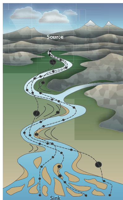
Figure 1 | The concept of a sediment-routing system. Sediment is transferred from a source region to a sink along trajectories shown by the dashed lines. Some trajectories involve short transit times with brief periods of storage in the sediment-routing system (small circles) (for example, on the river-channel bed), whereas others involve long transit times with prolonged periods of storage (large circles) (for example, in bars and flood plains). Storage of sediment implies buffering of incoming sediment flux signals.
