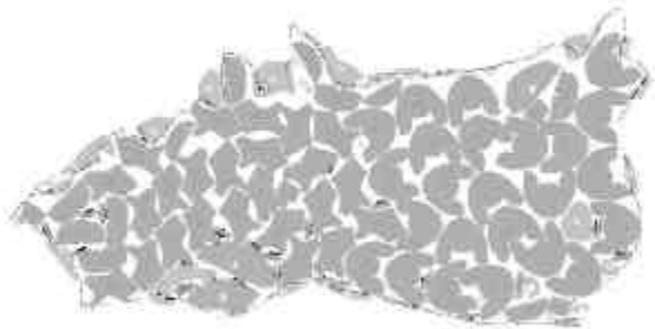
Figure 2: Leather nesting using the algorithm. Total waste is 21.0%
