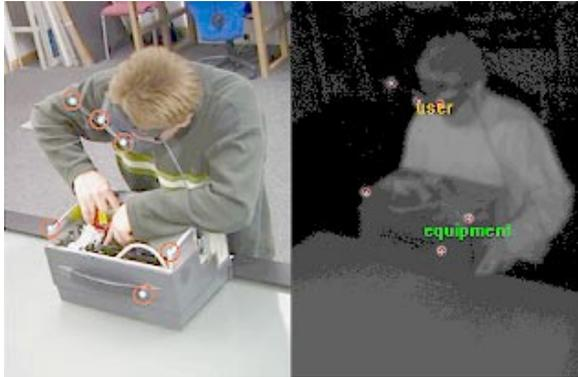
**Figure 4: View on tracked person and object from a normal camera and the infrared camera**
