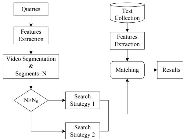
Fig. 2.1. The flowchart of CBCD system 2008.
