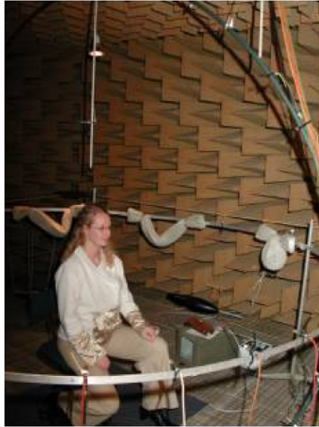
Fig. 4. The setup used for the directivity measurements of the soprano singer in an anechoic chamber.
