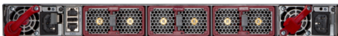
Arista 7280R3 1RU Rear View: Front to Rear airflow (red) AC Powered
