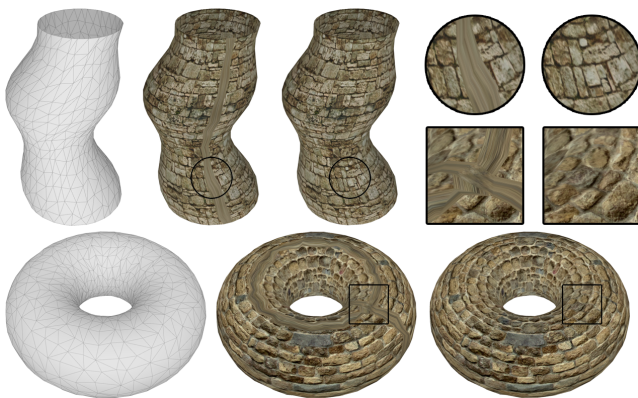
Figure 3: Toroidal/Cylindrical Textures: Traditional texture mapping (shown on the left side) reveals the seams. Toroidal/cylindrical mapping [Tar12] (shown on the right) eliminates the seams. Circular and square insets show close-ups.
