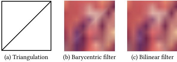
Figure 6: Mesh colors on (a) two triangles that form a square filtered using (b) a barycentric filter near diagonal edges, revealing the diagonal edge without causing discontinuity, and (c) a bilinear filter that filters across the diagonal edge.
