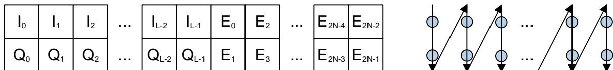
Figure 12A: IQ sample with mantissa-exponent uplink IQ data format
