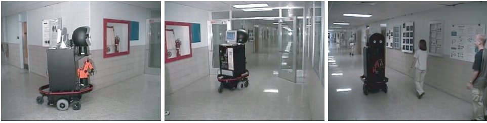
Fig. 12. The SAIL robot navigated autonomously using its vision-based sensorimotor skills that were acquired through online real-time developmental learning. It perceived the scene from its video cameras without using any range sensors.
