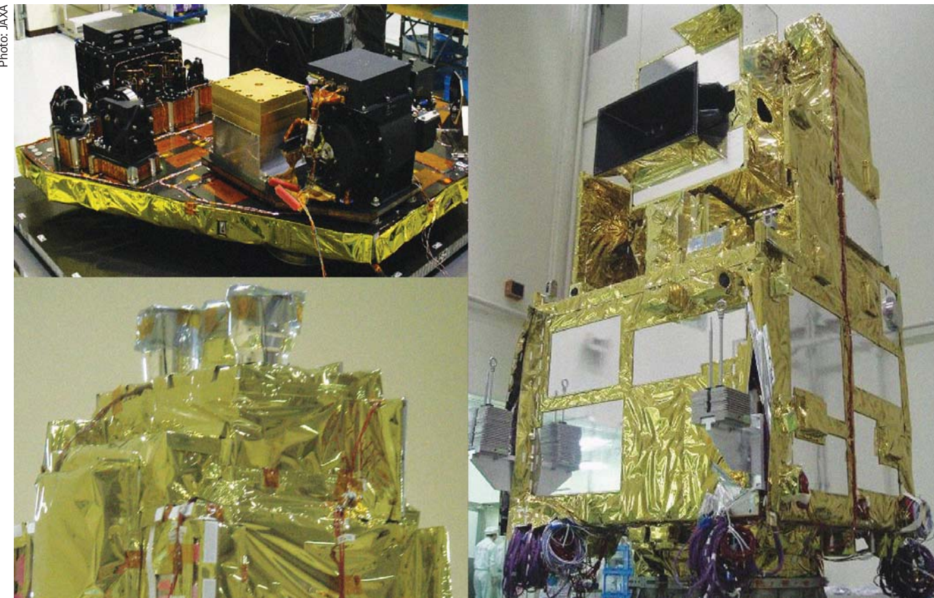
Top left: Thermal and Near Infrared Sensor for Carbon Observation — Fourier Transform Spectrometer (TANSO-FTS) Engineering Model. Bottom left: Thermal and Near Infrared Sensor for Carbon Observation — Cloud and Aerosol imager (TANSO-CAI) Engineering Model. Right: Structure and thermal model
