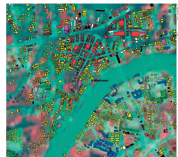
E-Flood Map, comprising flood maps derived from satellite data, the GIS database, and high-resolution satellite images
