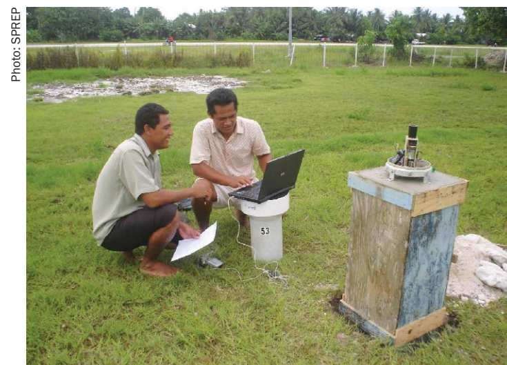
Installation of tipping-bucket rain gauge on Funafuti, Tuvalu
