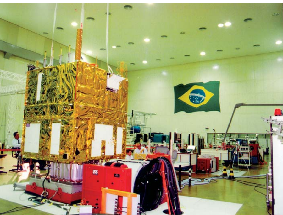
CBERS satellite being integrated and tested at INPE's assembly facility
