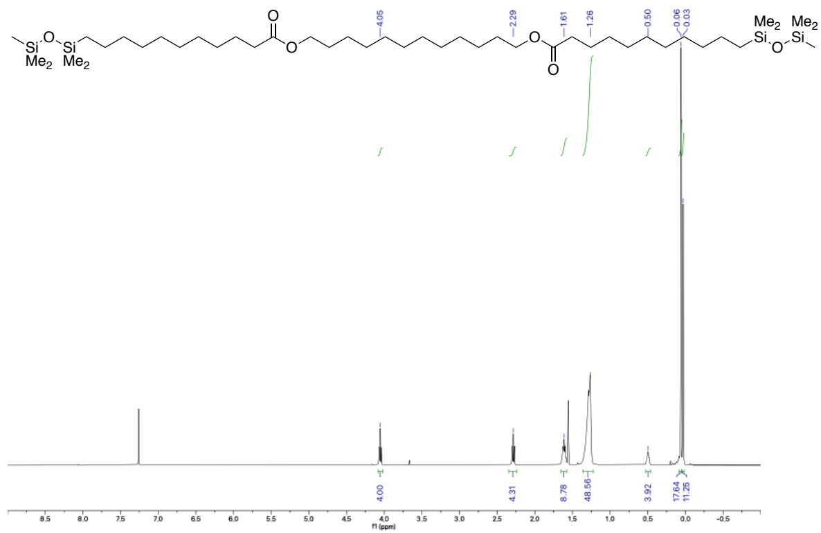
Figure 2.12.8.30. 1 H NMR spectra of compound 9 after depolymerization in the presence of PET, PP, and PE
