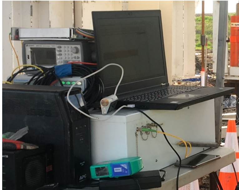
Figure 3-8: ALICIA fiber optic analyzer during load test
