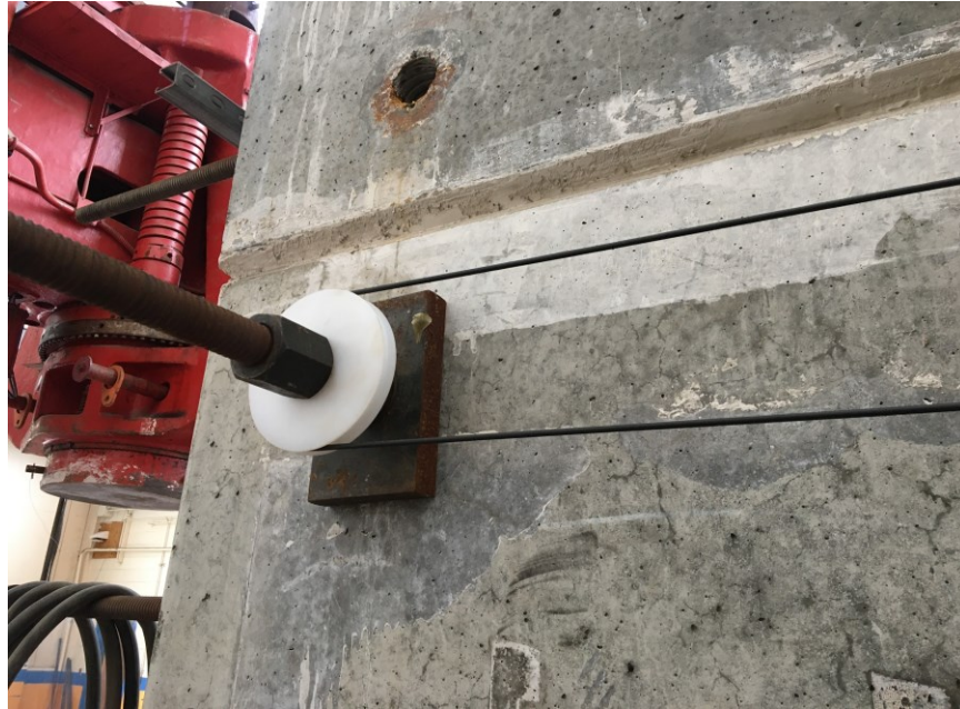
Figure 3-16: Photo of Loop 2 (long loop) pulley mounted on strong wall
