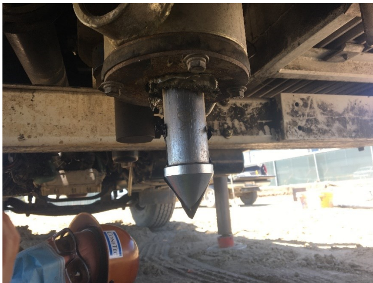
Figure 5-32: Dummy cone taped in place at the bottom of the first CPT rod
