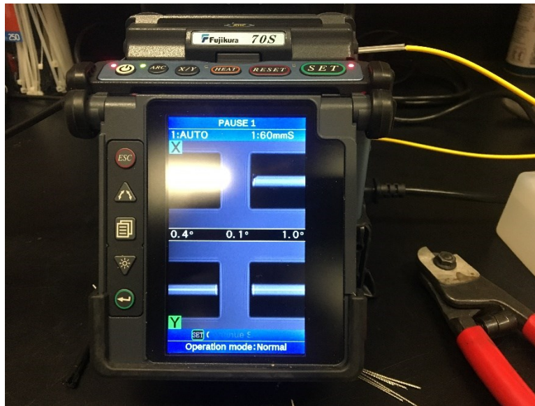
Figure 4-23: Fujikura fusion splicer, joining strain cable (left) and FC patch cable (right)
