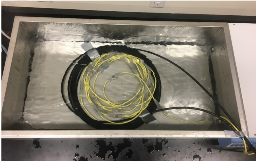
Figure 3-11: Photograph of the cable configuration within the water bath.
