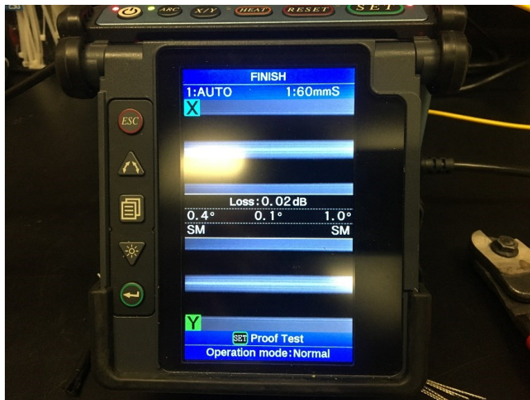
Figure 4-24: Photo of completed splice between strain cable (left) and FC patch cable (right)
