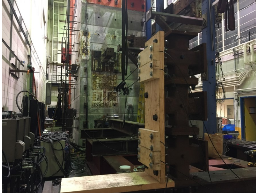
Figure 3-17: Photo of wood clamp setup at far corner of 1D shake table
