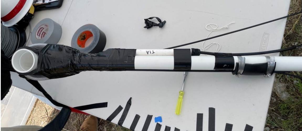
Figure 5-5: Fiber optic cable turnaround detail
