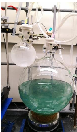
4. Transfer the ozonolysis solution to the copper mixture (the end)
