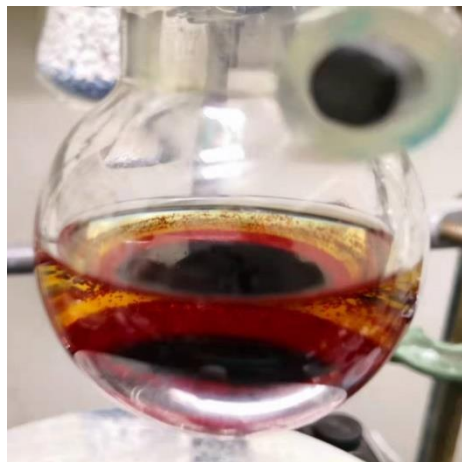
Recrystallization by layering a THF/DMSO solution with Et 2 O
