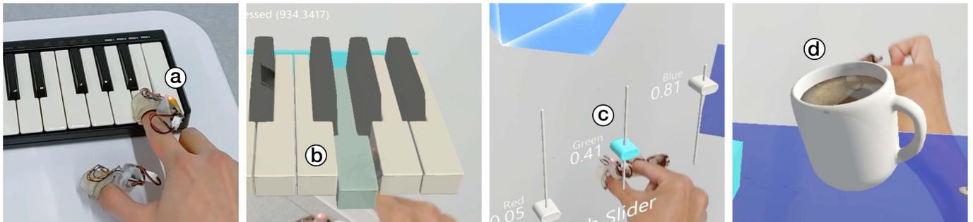
Figure 5: Adding contact haptic feedback to GUI widgets in existing Microsoft HoloLens Mixed Reality Toolkit (MRTK) while preserving the ability to feel physical objects: (a) pressing a physical piano key (b) pressing a virtual piano key (c) pinching a slider, (d) grabbing objects, a coffee mug in this case.
