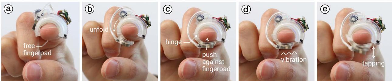
**Figure 2:** (a) When not in use our device keeps the fingerpad free for feeling the haptics of real-world objects. When activated, it unfolds (b) via a rack and pinion, and (c) a hinge redirects the force against the user’s fingerpad, which allows it to create three types of haptic effects: contact (pressure of the cover), (d) high-frequency textures (using an LRA embedded in its cover), and (e) low-frequency textures (by rocking the cover back and forth).
