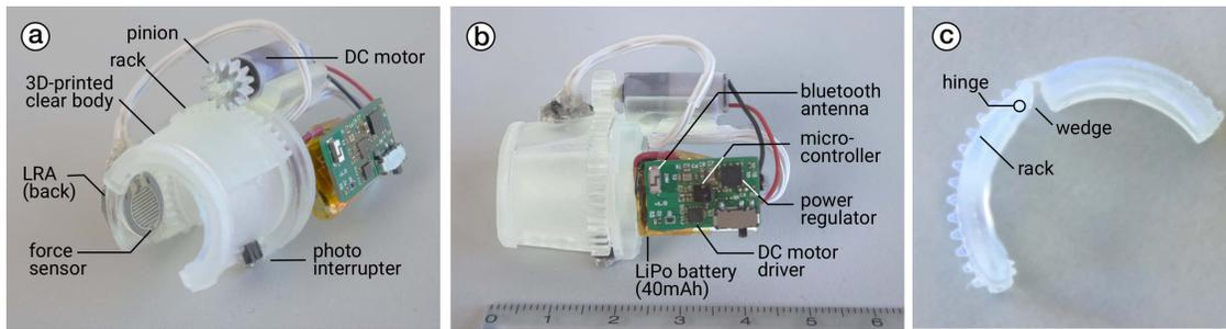
Figure 3: (a) Our self-contained haptic device; (b) detail of its cover; (c) top view of our device with ruler unit in cm.
