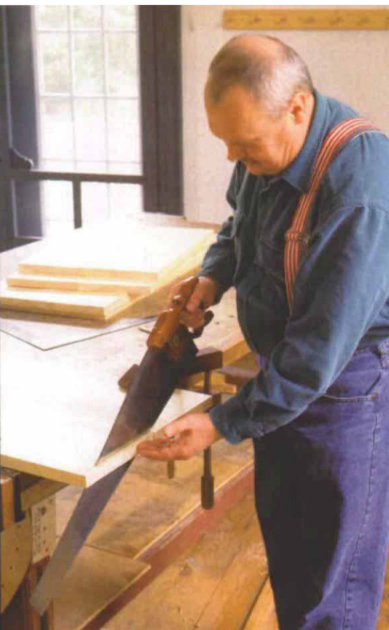
Two-handed bandsawing. To avoid breaking a fragile edge, and thus making it difficult to restart a cut, hold the fingertips of your free hand lightly against the thin waste piece. To saw a square edge, stand directly above the cut so that you see the thin top edge of the saw, rather than either side of the blade.
