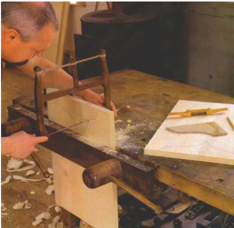
Bowsawed bootjack. A plywood half pattern, seen on the uncut panel, is used to trace the bootjack end that forms the blanket chest's feet. If the bowsaw jams in the cut, pop out the waste piece with a chisel blow to the panel's end grain.
