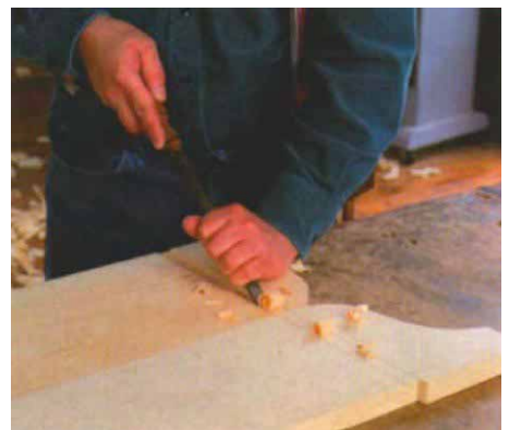
Scribe with a knife, then cut a dado with a chisel. Soft white pine, used for this chest and for thousands of similar antique versions, cuts easily with sharp hand tools. After a little chisel work, scribe again with the knife to cut cross-grain fibers until the dado is 1/2 in. deep.
