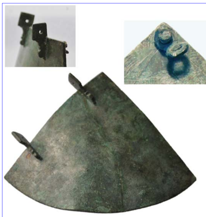
Fig. 5. Photographs of the back of the quadrant, the sights, and the swivel fixing for the plumb-bob. 1
