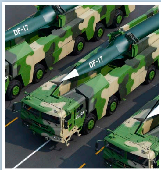
DF-17 Medium Range Ballistic Missile (MRBM), which is viewed as being capable of carrying a Hypersonic Glide Vehicle (HGV) [Avalon/Jiji Press Photo]
