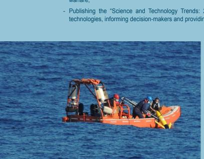
Centre for Maritime Research and Experimentation researchers deploying a Slocum Glider equipped with innovative sensing technologies during the Mediterranean-Recognized Environmental Picture 2020. Sicily Channel, Italy, October 2020.
